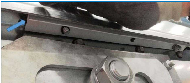
Installed sealing profile
