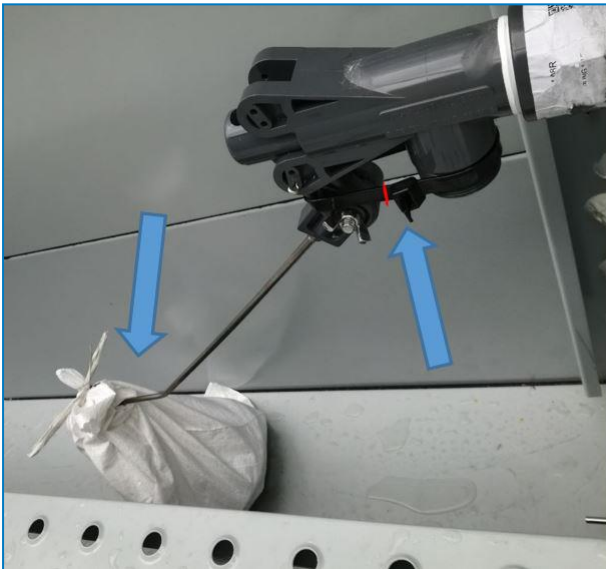
Fixation and wrapping of float ball
