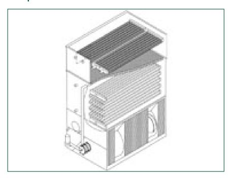
Ammonia (R-717) reciprocating compressors give off highly superheated gas, which should be **cooled** via the desuperheater coil before it enters the condensing coil.
