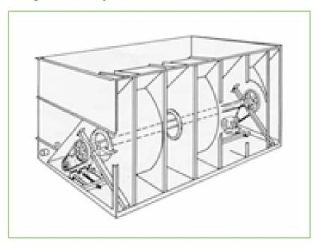
The installation of a Baltiguard® drive system
